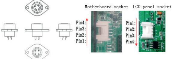
1. The motherboard socket: Pin1 to 12V+, Pin2 to B, Pin2 to A and Pin4 to GND.
