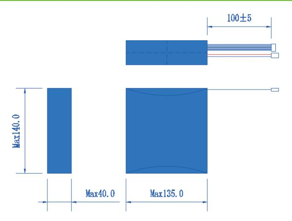
Note: PH2.0-5P white ribbon cable leakage length to  $100\pm 5$  mm. XT60 banana plug exposed by the terminal for actual length shall prevail
